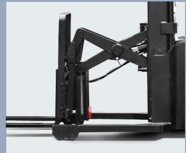
Forks move forward by the scissor structure
