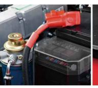
Integral locking pin structure on the baseboard can be opened without tool, which is convenient for daily repair and maintenance.
