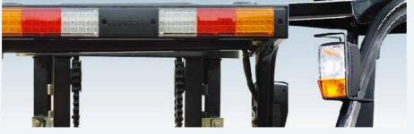
The new efficiency lighting system employs LED illuminant and new type reflector to reduce energy consumption, improve significantly illumination performance and prolong work time.
