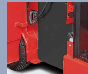
The battery can be removed from truck side, so it is very convenient for battery maintenance
