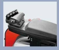
A series of high-performance version equipped with Fingertip control on seat armrest, which can be four positions adjusted to meet different operator' sdemands, release operator fatigue. Emergency switch, horn, fingertip control levers are all centralize on the armrest, which via CAN bus connection, provide good reliability.
