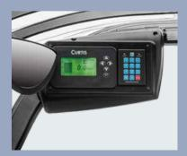
Easy to see dashboard is relocated to overhead, no restriction of the operator's visibility. The forklift is also applied PIN code access for better management.
