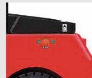
Forward/Reverse inching switch and emergency switch are mounted on the left rear, them make the hook easy and safe
