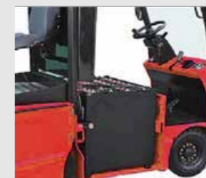
Side change battery design is convenient for changing battery
